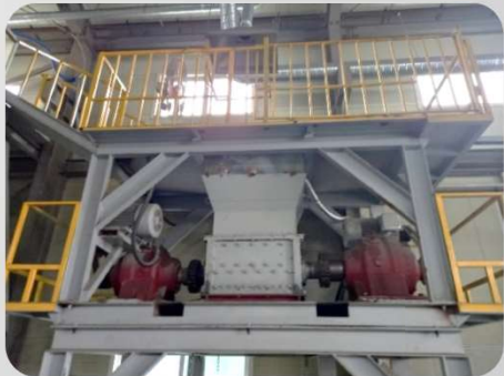
Double Shaft Shredder
