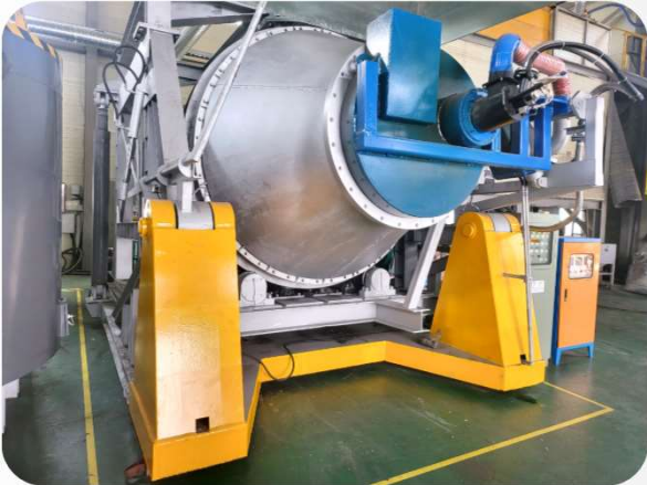
Rotary Furnace (8t/Chg.)
