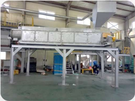
Rotary Kiln for Coating Removal
