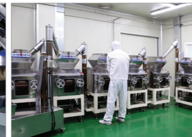
04 _ Grinders (iron powder removal)
