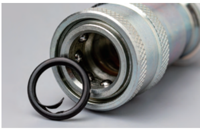
Frequent rubber hardening damage of valve O-Ring
